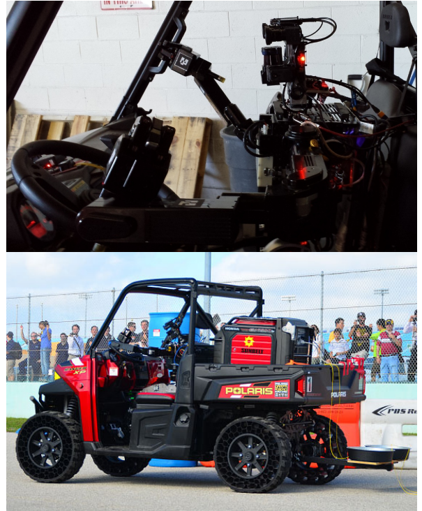
Fig. 1. DRC-Hubo in Polaris vehicle. (Top) Close-up during indoor testing; (bottom) At 2013 DARPA DRC trials (image courtesy of IEEE Spectrum Magazine)
