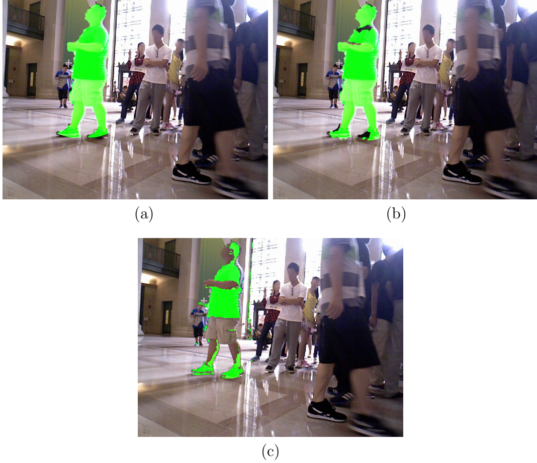
Figure 5.12: The results of GC-Refine-Pre for a given same input image. (a) shows the refinement result, if only the depth data is used, (b) displays the result of combining the normal and the depth of the points, (c) shows the refinement produced by combining RGB color, the normal, and the depth of the points. It can be realized that these combinations of the cues produced best three overlapping scores in Table 5.3.
