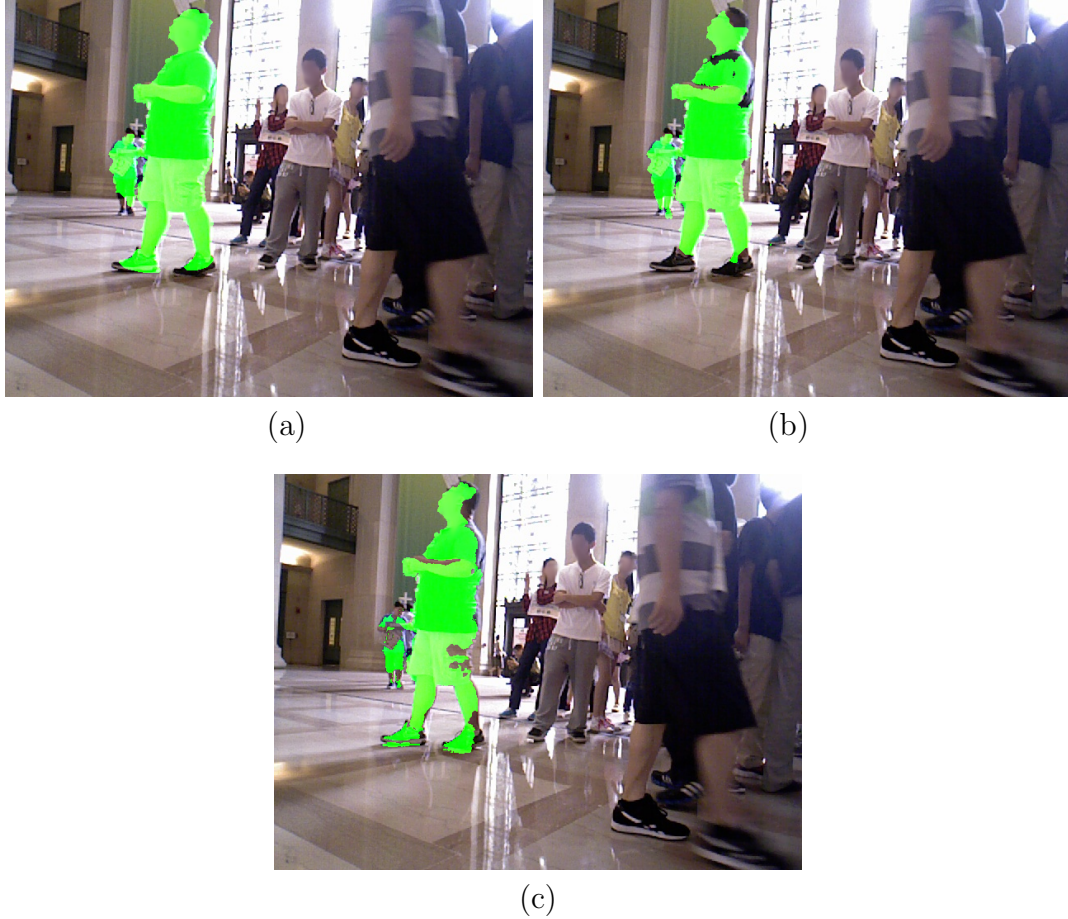
Figure 5.11: The results of GC-Refine for a given same input image. In this case, the distance cue is incorporated into all different combinations of the cues by default. (a) shows the refinement result, if only the depth data is used, (b) displays the result of combining the normal and the depth of the points, (c) shows the refinement produced by combining RGB color, the normal, and the depth of the points. It can be realized that these combinations of the cues produced best three overlapping scores in Table 5.2.
