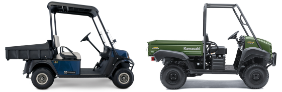
Fig. 5. Sample utility vehicles (Cushman Hauler and Kawasaki Mule) from set used to learn vehicle dimensions. Note the different heights and widths of the floor step areas and locations and angles of the steering wheels.
