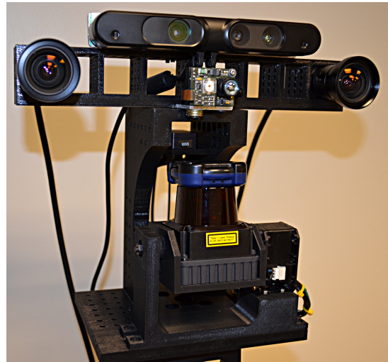
Fig. 2. Prototype sensor head with Asus Xtion Pro Live and tilting Hokuyo UTM-30LX-EW. Stereo color cameras, a PMD CamBoard nano, and a Microstrain IMU are also included but not used here.
