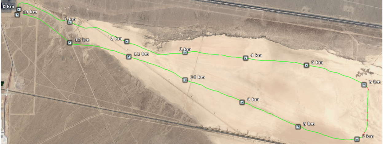
Fig. 12. GPS log of Alice’s GCE 2005 race. Markers at 1 km intervals show the directionality of the course. Green locations were classified as road and red as non-road (with a -0.1 confidence threshold). The area shown is roughly 6.2 km by 2.4 km; north is to the right (image courtesy of Google Earth)
