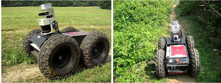
Fig. 1. Our robot autonomously following flat and thickly vegetated trail segments (see text for definitions)
