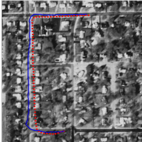
Figure 3.8: Using texture-driven dynamics and model-switching (not shown) with highly inaccurate GPS (red) positions. Solid blue curve shows corrected path
