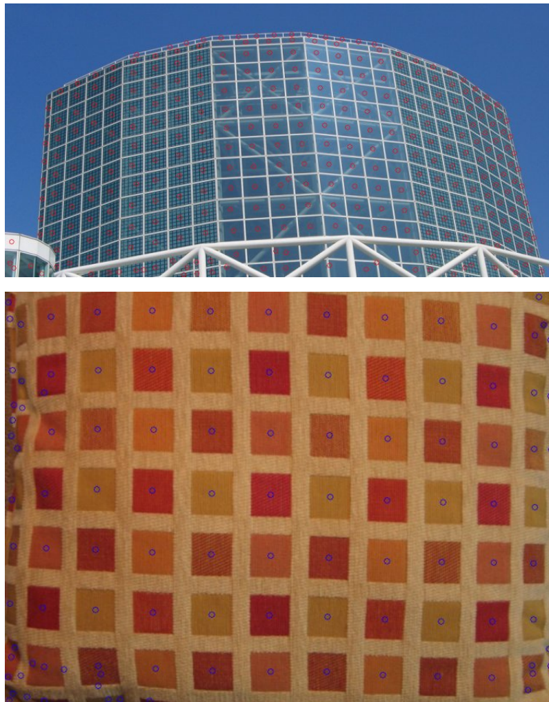
Figure 5.19: MSER features (shown as red or blue circles) detected for two images.
