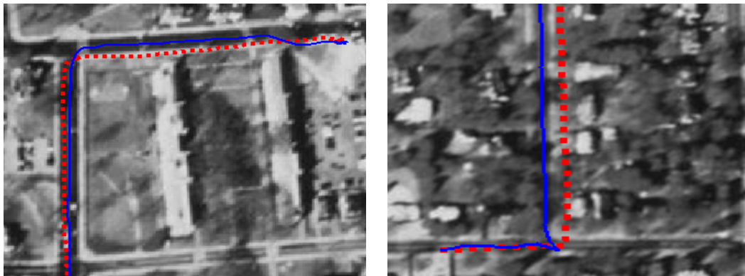
Figure 3.7: Corrected GPS positions (solid blue) at intersections. GPS estimates (dotted red) were especially inaccurate at intersections.
