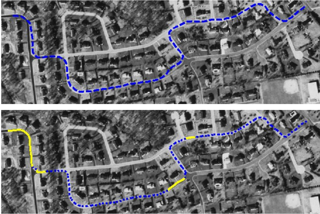
Figure 3.6: Comparison of single-mode and mixed-mode tracking using models M_1 (dark roads) and M_2 (bright roads). Solid yellow indicates that the tracker is in mode M_1 and dashed blue denotes M_2 . Notice how tracking only with M_2 causes mistracking on the darker roads.
