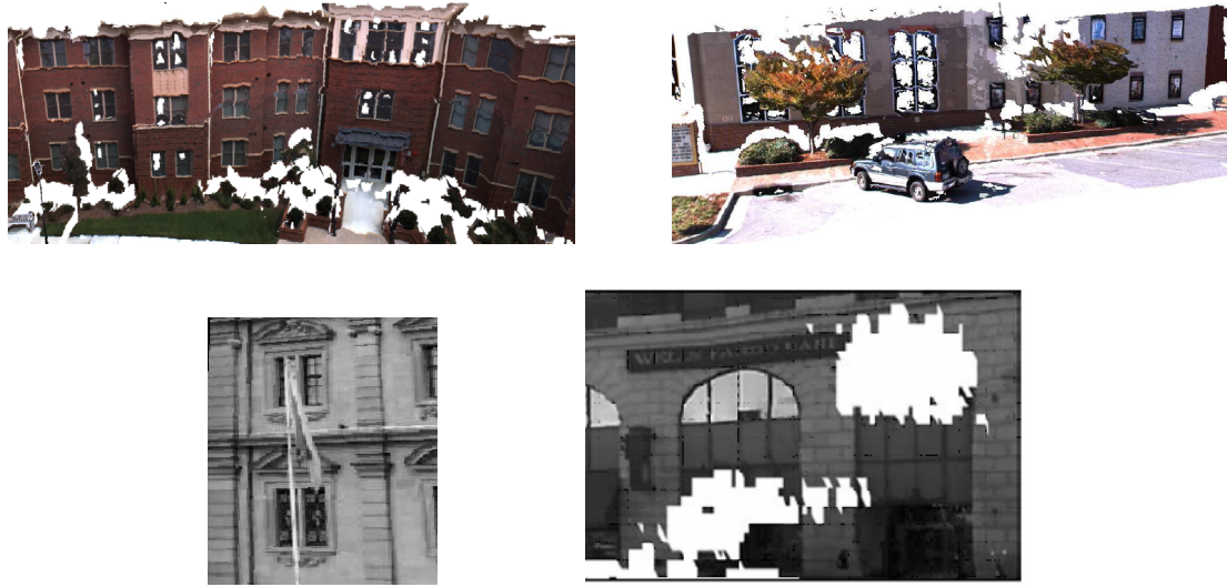
Figure 1.2: Some textured models from the UrbanScape Video Modeling project at UNC (top row), F. van den Heuvel’s project (bottom-left) at the Delft University of Technology [164] and the 3D City Modeling project at Berkeley (bottom-right) [49]. Foreground objects either cause holes in the model or appear pasted on the texture map.
