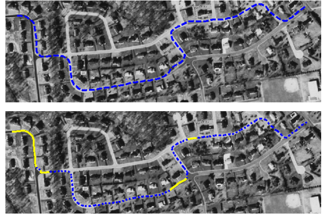
Fig. 3. Comparison of single-mode and mixed-mode tracking using models M_1 (dark roads) and M_2 (bright roads). Solid yellow indicates that the tracker is in mode M_1 and dashed blue denotes M_2 . Notice how tracking only with M_2 causes mistracking on the darker roads.
