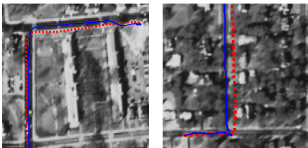
Fig. 4. Corrected GPS positions (solid blue) at intersections. GPS estimates (dotted red) were especially inaccurate at intersections.
