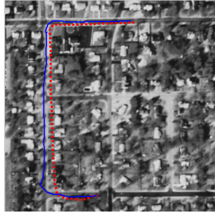
Fig. 5. Using measurement likelihood-driven dynamics and model-switching (not shown) with highly inaccurate GPS (red) positions. Solid blue curve shows corrected path
